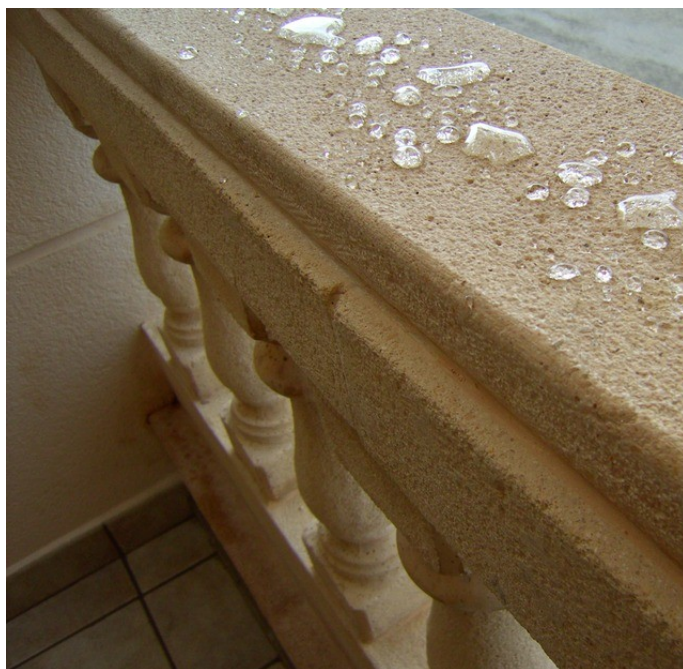
Beading and water-repellent effect on natural stone
